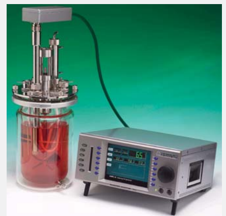
Biomass monitor 220 (Aber Instruments Ltd., UK) for real-time measurement of viable cell concentration. Photograph shows a cell culture application with a top entry electrode.
