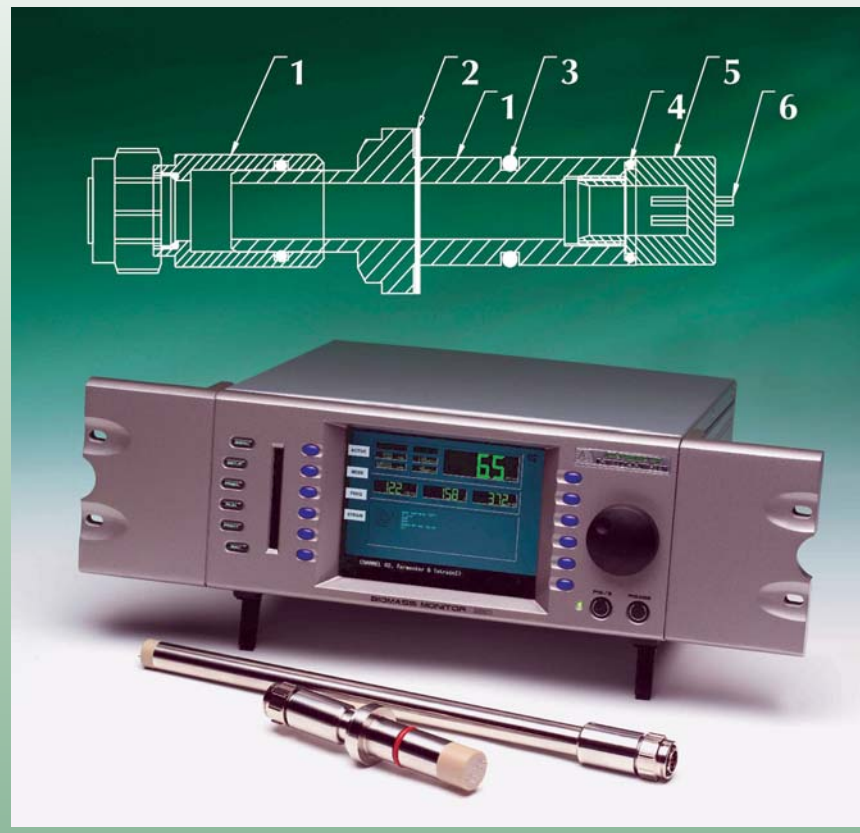
Figure 2: Biomass Monitor 220 (Aber Instruments, Ltd., UK) with 25-mm and 19-mm diameter probes. Materials of construction for the 25-mm probe: (1) probe body, 316 stainless steel; (2) neoprene sealing washer; (3) port O ring, FDA-approved silicone; (4) internal O ring, FDA-approved nitrile; (5) probe tip, Victrex PEEK approved to FDA 21 CFR 177.2415 for repeat food contact (meets the requirements of USP class VI); (6) electrode pins, 99.99% FDA-approved platinum.
